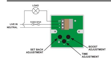
Wire the ENERSTAT-T as in the diagram.
