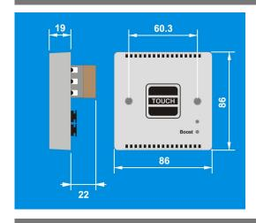
The ENERSTAT-T electronic thermostat will accurately maintain the temperature of a room at two levels (or setpoints): the setback temperature and the boost temperature.
